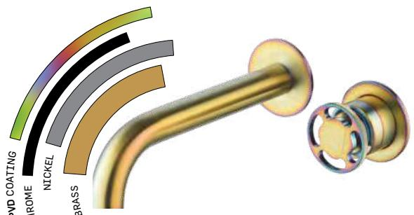
Is a thin ceramic coating with high adhesion, performed in a highly ionized plasma deposition process in a vacuum chamber, where temperatures can range from 60° to 500°C. The high temperatures allow for **coatings with high purity**, being **chemically inert and biocompatible**.
